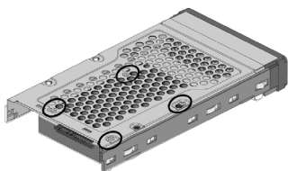
Figure 2-13-1. Installing 2.5-inch SAS/SATA Drive
