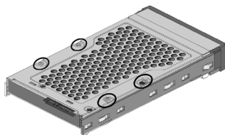
Figure 2-13-2. Installing 3.5-inch SAS/SATA Drive
