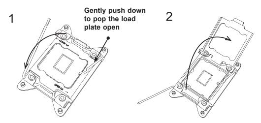
4. Use your thumb and index finger to hold the CPU on its edges. Align the CPU keys, which are semi-circle cutouts, against the socket keys.
