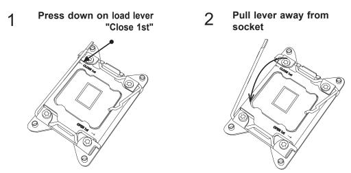
3. With the "Close 1st" lever fully retracted, gently push down on the "Open 1st" lever to open the load plate. Lift the load plate to open it completely.
