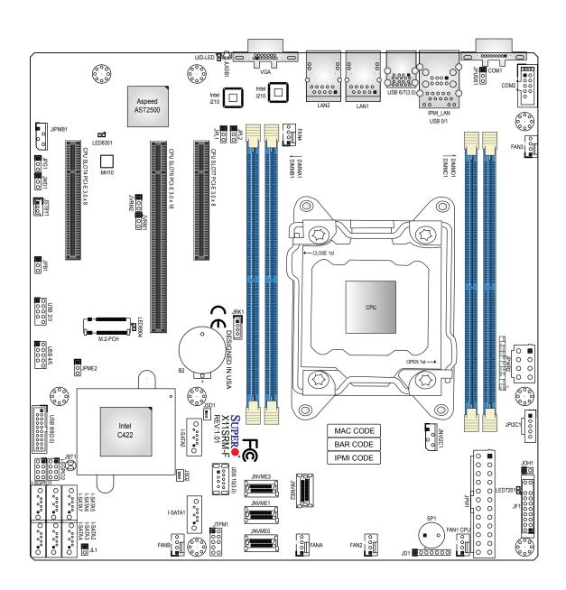
Figure 1-3. X11SRM-F/-VF Motherboard Layout (not drawn to scale)
