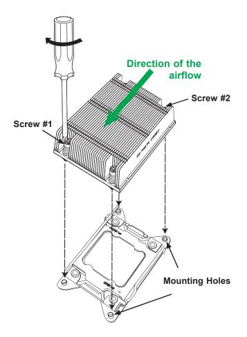
**Note:** For optimal airflow, please follow your chassis airflow direction to correctly install the CPU heatsink. Graphic drawings included in this manual are for reference only. They might look different from the components installed in your system.
