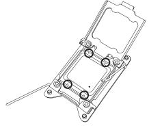
7. Close the load plate with the CPU inside the socket. Lock the "Close 1st" lever first, then lock the "Open 1st" lever second. Gently push the load levers down to the lever locks.
