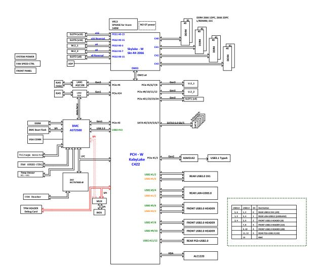
Figure 1-3. Chipset Block Diagram
