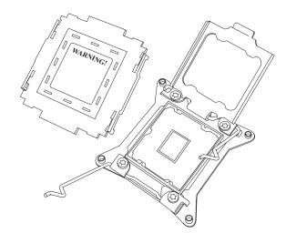
5. Use your thumb and index finger to hold the CPU on its edges. Align the CPU keys, which are semi-circle cutouts, against the socket keys.
