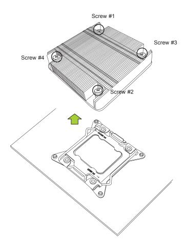
4. Once the heatsink is loosened, remove it from the motherboard.
