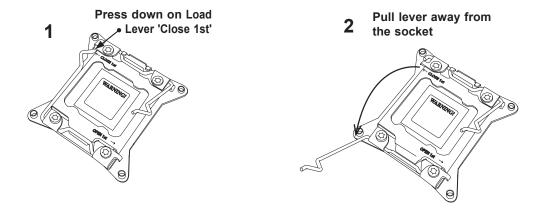
3. With the "Close 1st" lever fully retracted, gently push down on the "Open 1st" lever to open the load plate. Lift the load plate to open it completely.
