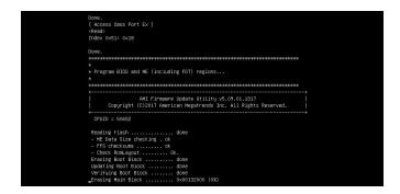
10. The screen above indicates that the BIOS update process is completed. When you see the screen above, unplug the AC power cable from the power supply, clear CMOS, and plug the AC power cable in the power supply again to power on the system.
