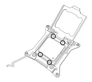
8. Close the load plate with the CPU inside the socket. Lock the "Close 1st" lever first, then lock the "Open 1st" lever second. Gently push the load levers down to the lever locks.
