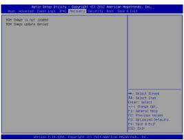
4. After locating the new BIOS binary image, the system will enter the BIOS Recovery menu as shown below.
