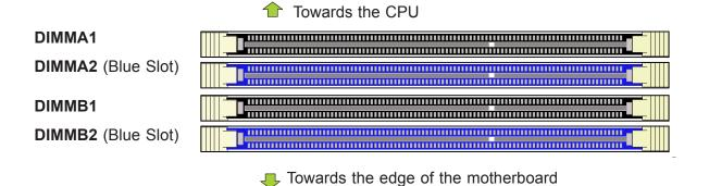
**Note:** Be sure to use memory modules of the same type and speed on the motherboard. Mixing of memory modules of different types and speeds is not allowed.
