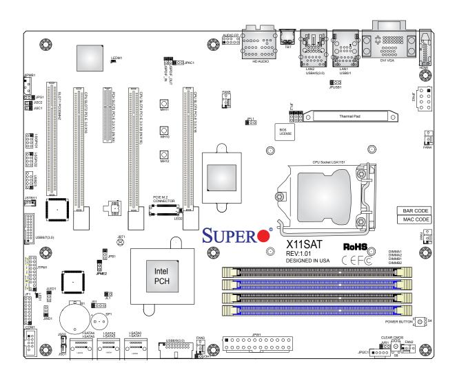
Figure 1-3. X11SAT/X11SAT-F Motherboard Layout (not drawn to scale)
