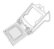
5. Do not rub the CPU against the surface or against any pins of the socket to avoid damaging the CPU or the socket.
