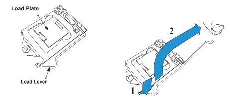
2. Gently lift the load lever to open the load plate. Remove the plastic cap.
