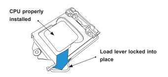
**Note:** You can only install the CPU inside the socket in one direction. Make sure that it is properly inserted into the CPU socket before closing the load plate. If it doesn't close properly, do not force it as it may damage your CPU. Instead, open the load plate again and double-check that the CPU is aligned properly.
