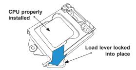
Attention! You can only install the CPU inside the socket only in one direction. Make sure that it is properly inserted into the CPU socket before closing the load plate. If it doesn't close properly, do not force it as it may damage your CPU. Instead, open the load plate again and double-check that the CPU is aligned properly.
