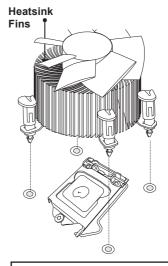
Recommended Supermicro heatsink: SNK-P0046A4 active heatsink
