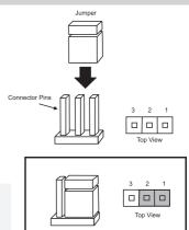
Connector Pins with a Jumper installed on pins 1 and 2.
