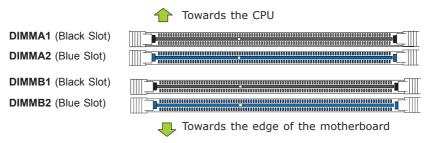
The X11SAE/X11SAE-F supports up to 64GB of Unbuffered (UDIMM) ECC/non-ECC DDR4 memory, up to 2133 MHz in four memory slots. Populating these DIMM modules with a pair of memory modules of the same type and same size will result in interleaved memory, which will improve memory performance.
