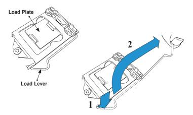
Gently lift the load lever to open the load plate. Remove the plastic cap.
